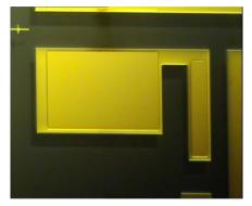
Using a lighter gas atmosphere is the next best option, and He the only practical safe solution, providing reasonably effective debris control. The photo at left indicates opening of contact areas to gold film; the width of the larger opened area here is approx. 1mm. Just a trace of redeposit can be seen between this zone and its neighbour above(out of the picture).
