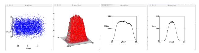
An early trick in excimer processing was to pass the beam through a weak **biprism**, cutting the beam in two & by refraction ensuring that the two halves converge & overlap on a downstream plane, here for the short axis. The match can be good enough to produce the desired **top-hat profile**:- N.B. This works less well for the long axis (right).
