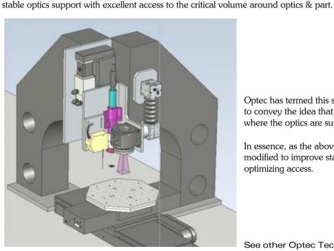
Optec has termed this system architecture a Space Frame to convey the idea that it rigidly fixes a point in space,-where the optics are supported.
