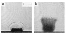
Some marking applications in polymers rely on thermal foaming of the material to generate contrast. This requires somewhat deeper absorption, at longer wavelength and longer pulse duration
