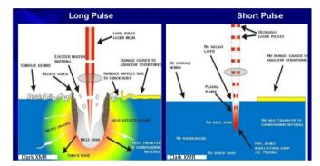
During a laser pulse of duration t, heat will travel distance on the order of sqrt(4 $\alpha$ t) where  $\alpha$  is the thermal diffusivity in cm<sup>2</sup>/s, equal to  $K/\rho C$ , and mainly determined by the thermal conductivity K. Thus, machining of fine features in thermally conducting materials absolutely requires short pulse duration. For ps/fs lasers, the thermal diffusion distance can be  $< 1\mu$ m.
