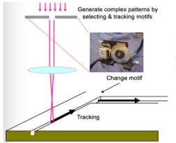
In an intermediate case, smaller fundamental motifs are projected and combined with part motion to produce larger or more complex motifs,- a combination of sequential/parallel processing. The most efficient method in any particular task depends partly on the task, and partly on the characteristics of the laser source. As always, the tool & technique must be chosen for the job in hand.
