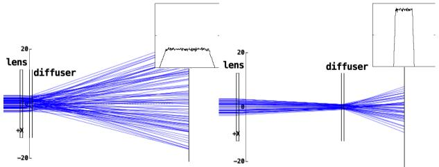
When used to illuminate the mask in a projection system with demagnification then one has to think about filling of the projection lens aperture, which is optimized in this arrangement: -
