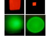
N.B. lens & diffuser can be placed in either order; if diffuser is placed after the lens and the former moved closer to the focal plane then the result is a smaller spot of higher intensity.
